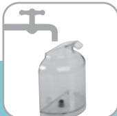
Empty, rinse and fill water tank with fresh water
