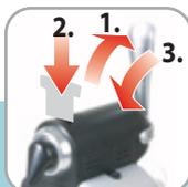
1. Lift lever, 2. insert filter, 3. close lever
